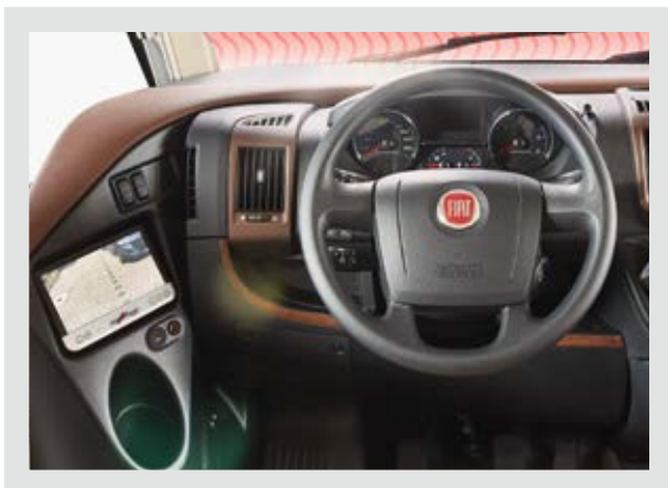
▲ Driving security: Clear and functional design. Targeted heating of the dashboard front prevents cold from being radiated from the windscreen, reversing camera monitor in a glare-free location
