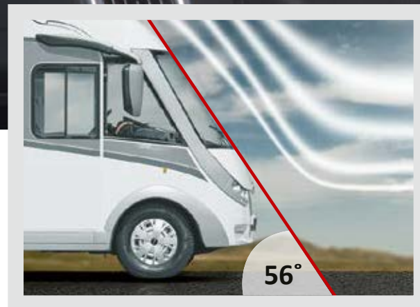
▲ Three-dimensionally shaped front with extra-flat angle = less air resistance, less fuel consumption and less wind noise
