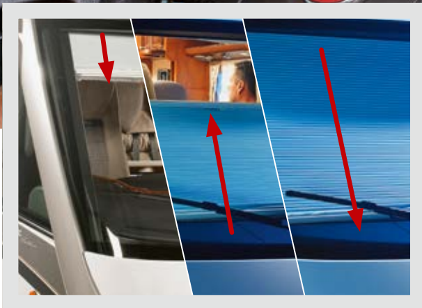
▲ Multi-functional insulating pleated windscreen blind , can be operated horizontally to simultaneously allow it to function as a sun blind, for privacy protection and as a blackout with insulation
