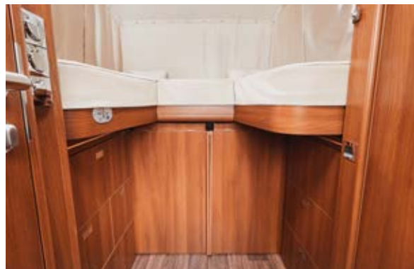
▲ Cold from the driver's cabin is sealed off underneath the fold-down bed when it is in the sleeping position
