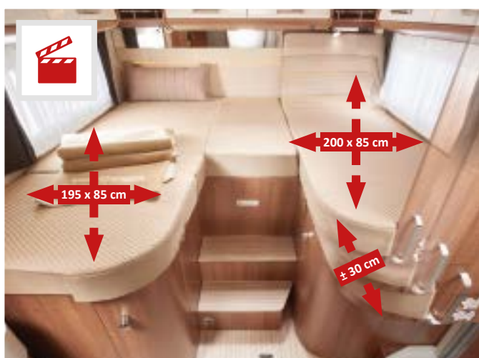
▲ Registered for patent approval: Single bed can be moved by 30 cm for comfortable living and sleeping conditions within a short vehicle length (I 144 LE)
