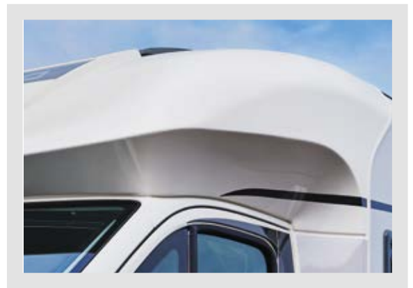
▲ Carthago front shroud: the Carthago front shroud combines elegant design and high-quality GRP structure. Thanks to the two shell insulation, the Carthago semi-integrated motorhomes provide the best living climate, even at low temperatures
