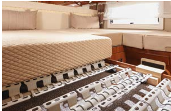
▲ Medically recommended, point elastic under-springing system in the rear bed
