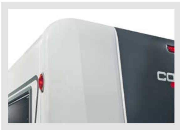
▲ The Carthago curved roof: a Carthago motorhome awakens emotions due to its unique and elegant design. The curved roof that is typical of the brand is such a design element. It also increases the torsion resistance of the body, and there is less susceptibility to side wind. The design and use are perfectly combined!
