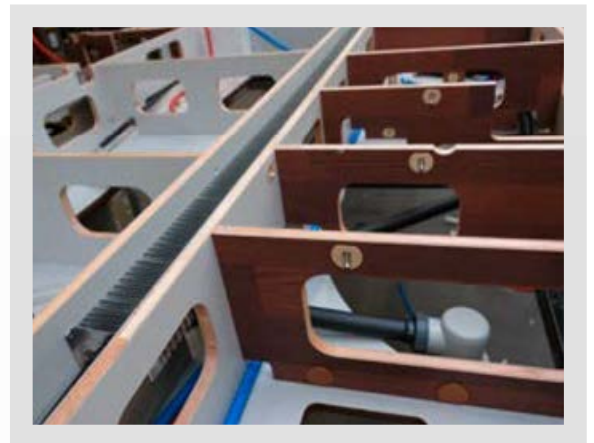
▲ The Carthago double floor Together with the high-stability self-supporting main body construction, it contributes to a providing high degree of stability and torsional rigidity, and is extremely lightweight at the same time. A "special light" AL-KO low frame is used exclusively for the lightweight models. Result: minimal weight and maximum ride comfort
