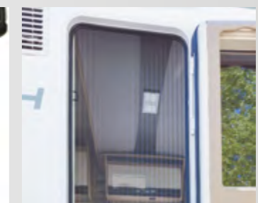
Entrance Door Pleated sliding mosquito net on entrance door. External LED light over the entrance door
